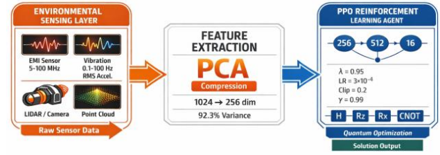
Figure 4. Adaptive PPO-QAOA Hybrid Feedback Control Architecture: Closed-Loop Quantum-Classical Navigation System with Real-Time Environmental Adaptation
