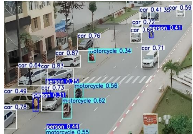
Figure 10. Visually display the results of small object detection using YOLOv11 and SAHI
