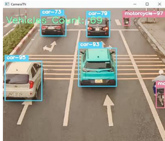
Figure 8. Examples of vehicle detection and tracking results using YOLOv11 and DeepSORT
