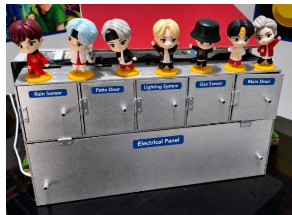
Figure 8. Three-dimensional control unit of the proposed prototype with integrated electrical panel and wiring
