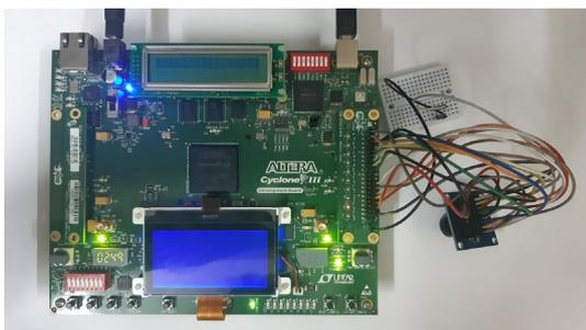
**Figure 15.** Real time implementation of the proposed sobel algorithm by interfacing the camera module with Cyclone III FPGA
