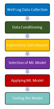
**Figure 1.** Methodology Process for the Identification of Lithology from Well Log Data using Machine Learning
