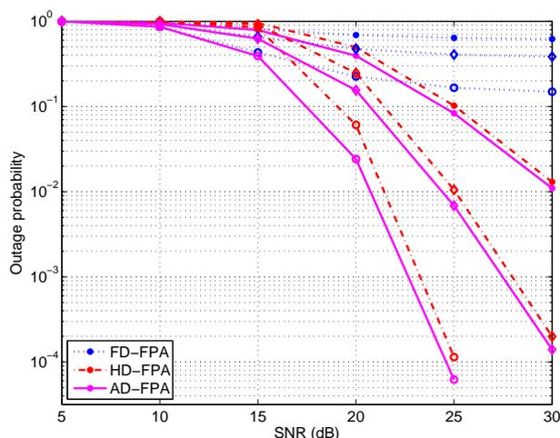
**Figure 3.** The outage performance of proposed schemes for cooperative NOMA, where  $R_1 = 0.5\text{bits/s/Hz}$ ,  $R_2 = 2\text{bits/s/Hz}$ , the power allocation factor  $\alpha_1 = \frac{3}{4}$  and the self-interference cancellation factor  $\kappa = 1$  (no cancellation technique) with relay numbers  $N = 2$ ,  $N = 4$ ,  $N = 8$ , respectively.
