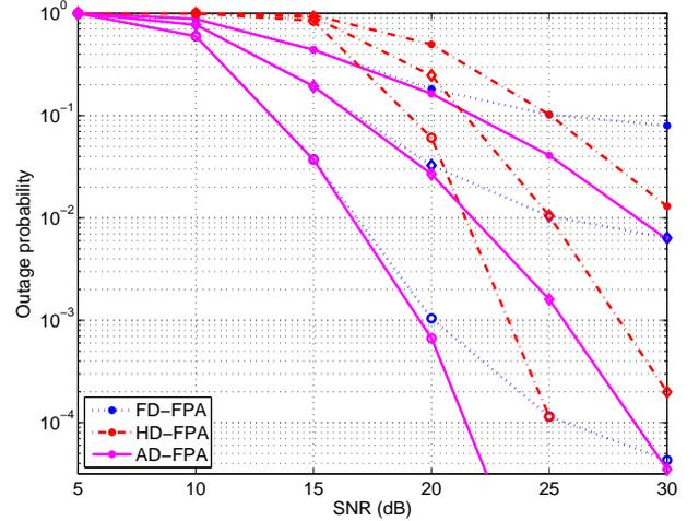
**Figure 2.** The outage performance of proposed schemes for cooperative NOMA, where  $R_1 = 0.5\text{bits/s/Hz}$ ,  $R_2 = 2\text{bits/s/Hz}$ , the power allocation factor  $\alpha_1 = \frac{3}{4}$  and the self-interference cancellation factor  $\kappa = 0.1$  with relay numbers  $N = 2$ ,  $N = 4$ ,  $N = 8$ , respectively.
