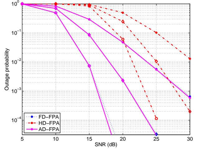
**Figure 1.** The outage performance of proposed schemes for cooperative NOMA, where  $R_1 = 0.5\text{bits/s/Hz}$ ,  $R_2 = 2\text{bits/s/Hz}$ , the power allocation factor  $\alpha_1 = \frac{3}{4}$  and the self-interference cancellation factor  $\kappa = 0$  (perfect cancellation technique) with relay numbers  $N = 2$ ,  $N = 4$ ,  $N = 8$ , respectively.
