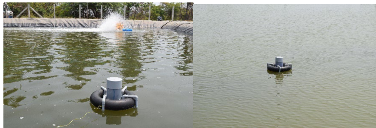
Figure 5. a) Aqua Buoys ready for deployment b) Testing in a small tub
