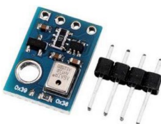
Figure 4. AHT10 temperature sensor
