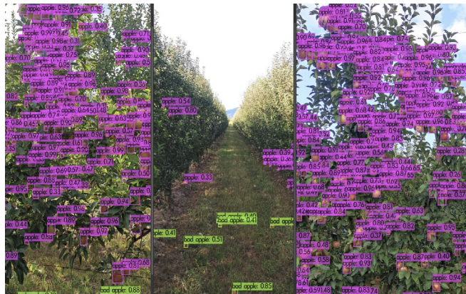
Figure 23. How the trained algorithm detects good and bad apples on frames.
