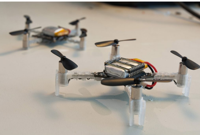
Figure 2. A miniature Crazyflie quadrotor. Crazyflie is an open source created for educational and research purposes [17]
