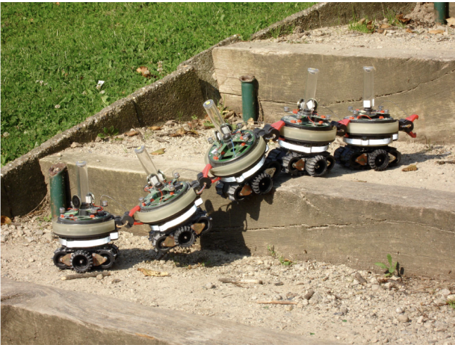
Figure 1. A Swarm-bots robots transgressing a challenging terrain. Robots are equipped with flexible grippers that enables them to connect with each other as demonstrated in the picture [15, 16]
