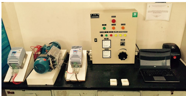
Figure 2. Installing the wind turbine system simulation bench: QTCM device and wind turbine simulation setup
