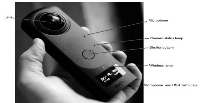
Figure 1. Key Specifications of the Ricoh Theta V Camera
