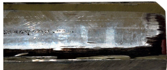
Figure 5. Tooth area (350...450 mm) showing the final traces of pitting (side B)
