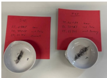
Figure 9. Pyrolysis analysis result for the filaments
