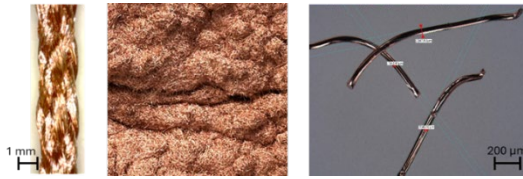
Figure 1. Copper fibers by AERUMTEC GmbH (Germany) produced out of a round braided copper (left) and subsequently cut and (middle) used in this research, (right) Microscopy photo from fibers
