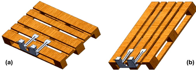
Figure 11. Pallet clamping: (a) by length; (b) by width [42]
