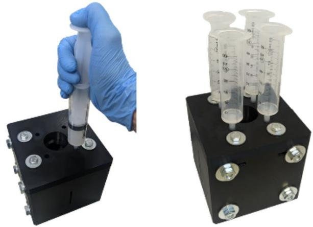
Figure 9. Process of filling the casting mold
