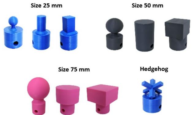
**Figure 5.** Examples of grip testing samples
