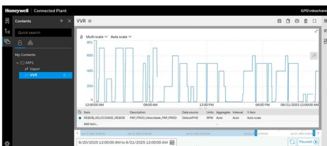
Figure 4. Dashboard view in Honeywell Uniformance showing the real-time speed graph of the rewinder machine.
