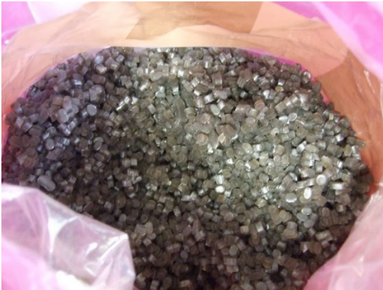
Figure 1 Recycled polyvinyl butyral (PVB) granulate prepared for additive manufacturing.
