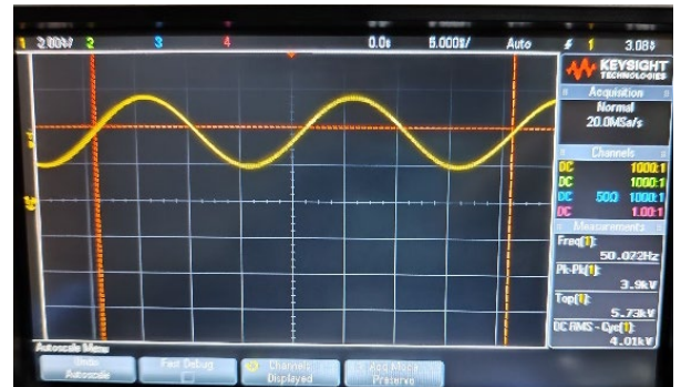
Figure 3. Waveform diagram of the AC/DC superimposed voltage
