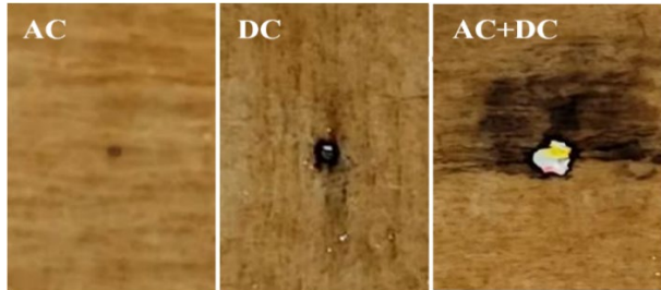
Figure 11. Surface morphology of oil paper insulation after breakdown
