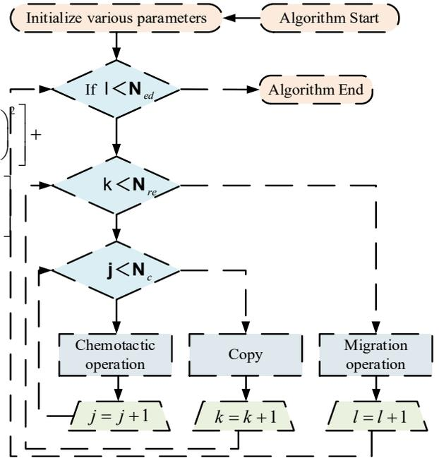
Fig. 2 Overall workflow of BFO algorithm
