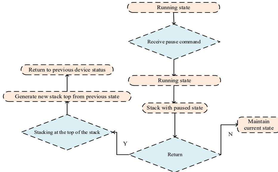
Fig. 4 Schematic diagram of intelligent equipment scheduling method based on stack
