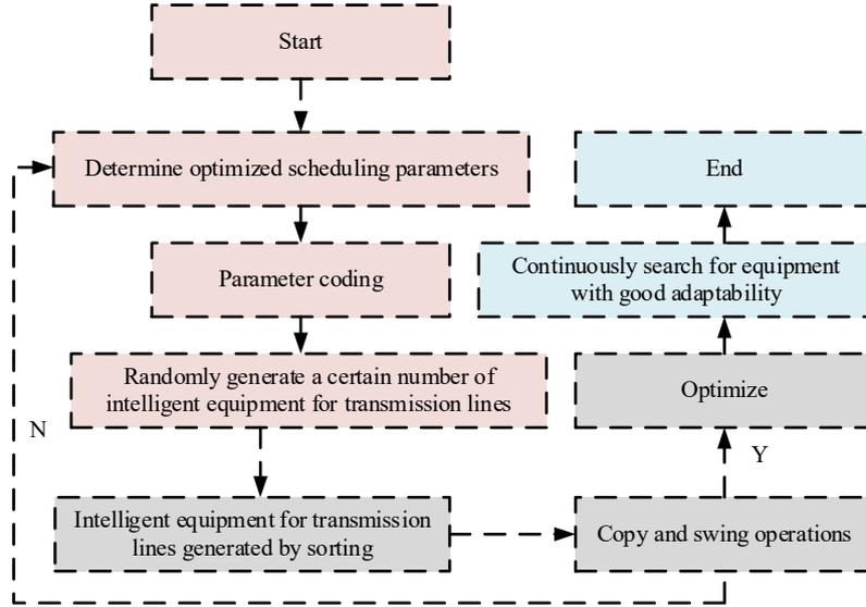
Fig. 6 Flowchart of Improved BFO Algorithm
