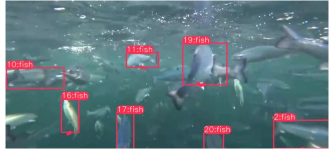
Figure 4. The detection performance of our YOLOv8-agri models on the screenshot of a fish farming. The number presents the unique object ID tracked by DeepSORT.
