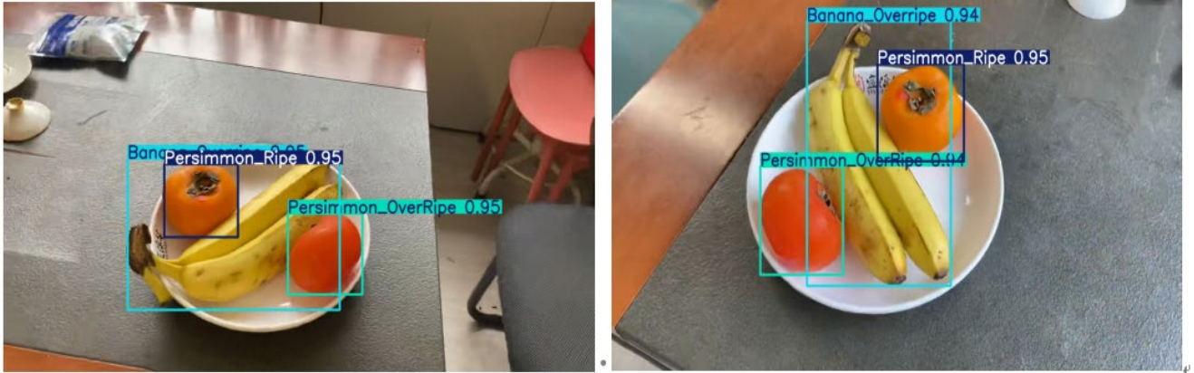
Figure 9. Multi-fruit detections under occlusion, clutter and specular highlights in real kitchens.
