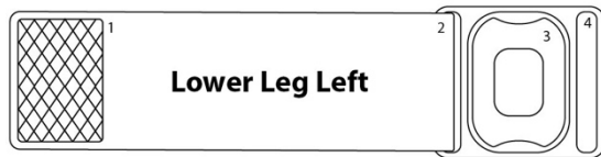
Figure 2. Design Sensor strap system: (1) Mushroom head Velcro fastener (2) One-sided Velcro bands made of neoprene with labeling (3) 3D-printed sensor case (4) Integrated opening in the sensor case serving as closure
