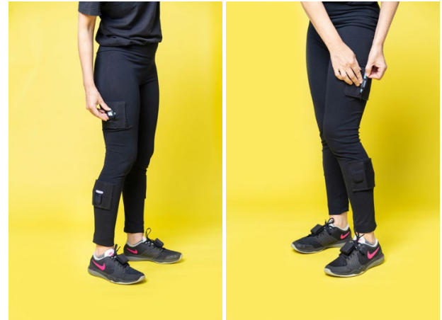
Figure 14. Two prototypes for pocket-based attachment methods for sensor integration: (1) the slide-in pocket, (2) zipper pocket
