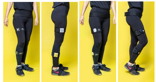
Figure 10. Four different prototypes of a strap-based sensor attachment system to explore various techniques and materials for sensor housings, closure mechanisms, size adjustability, and strap configurations
