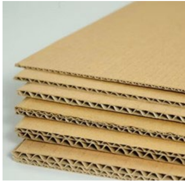
Figure 9. Corrugated-board layers used for panel selection
