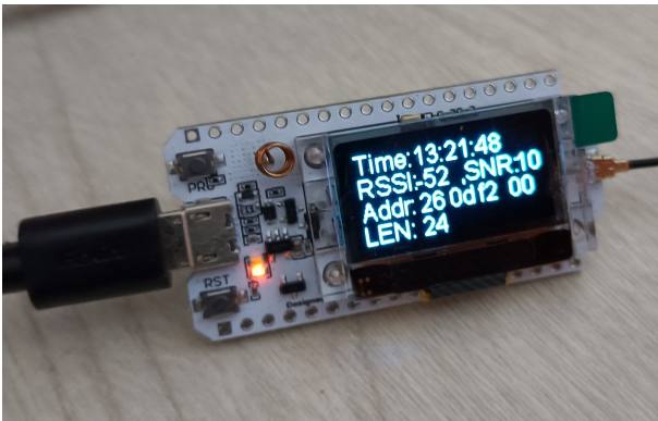
Figure 5. Board ESP32 - WiFi Lora 32 for Gateway LoRaWAN
