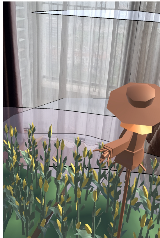
Figure 10. ARKit plane detection in Farmerly AR mobile app
