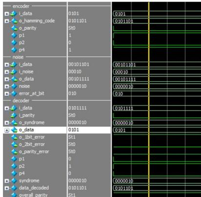
Figure 13. Output for one bit error
