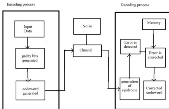
Figure 2. Block diagram for error detection and error correction
