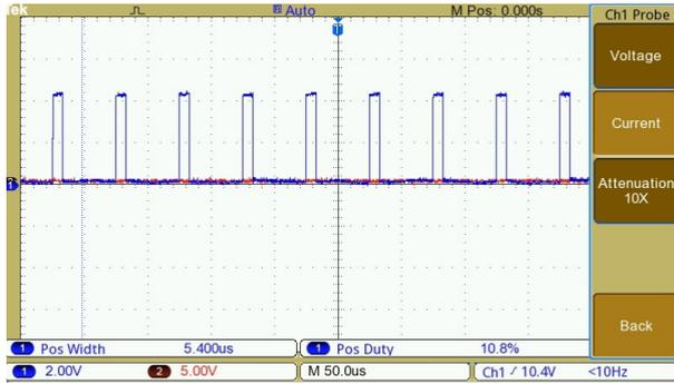
Figure 15. SEPIC Converter pulse at duty Cycle of 0.2
