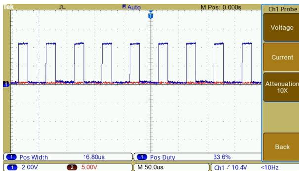
Figure 16. SEPIC Converter pulse at duty Cycle of 0.8
