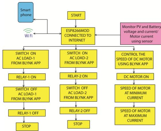
Figure 10. Block diagram for Blynk IOT server
