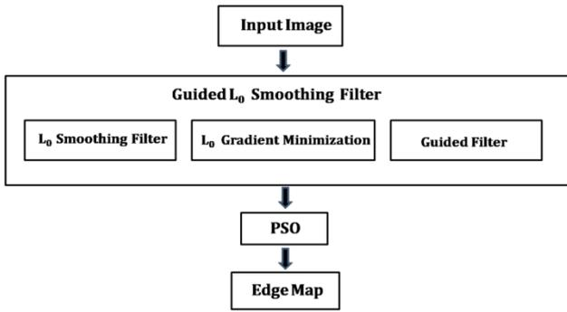
**Figure 2.** Block diagram for Guided L<sub>0</sub> smoothing filtering and PSO based edge detection process
