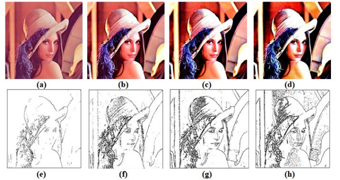
Figure 7. (a) Original Lena Image (b) 5% Sharpened Image (c) 10% Sharpened Image (d) 20% Sharpened Image (e) Detached edges original image (f) Detached edges 5% sharpened image (g) Detached edges 10% sharpened image (h) Detached edges 20% sharpened image
