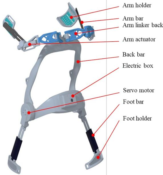
Figure 1. The architecture of prototype exoskeleton.
