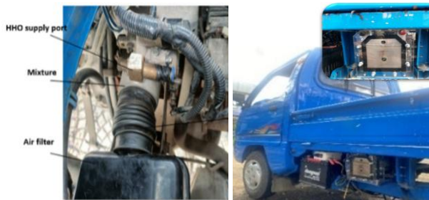
Figure 12. Installation of the venturi mixer and layout of the HHO electrolyser on the Thaco Towner 750 vehicle
