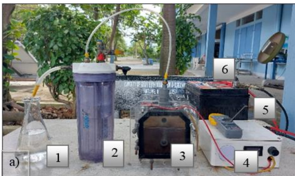
Figure 8. Experimental setup for measuring HHO gas flow rate
